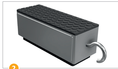
2 Test weight ready for measurement.
